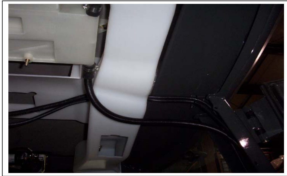
Left rear drain tube
